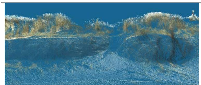
Figure 2 3D TLS data of sand dune
