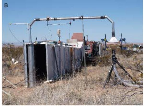
Figure 2: A) Landscape and vegetation of the study site B) Portable field wind tunnel deployed on a clipped (unburnt) shrub (SC) plot.
