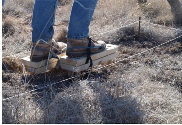
Figure 3: View of the trampling shoes detailing construction and picture of the clipped grass plots being trampled.
