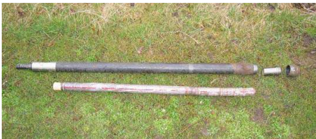
Figure 37 Core catcher sampler with core in sleeve
