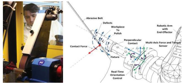
**Figure 2.** Manual polishing approached replicated on a robotic arm.
