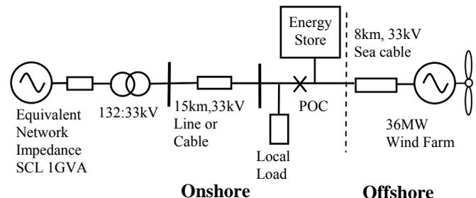
Fig. 1. Case study scenario 1: 36MW wind farm connecting to grid via a constrained 15km 33kV line. Assumed Local Load: 1.5 MW min, 4.5MW max.
