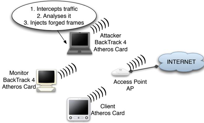
Fig. 3. Testbed and steps of attack for Airpwn
