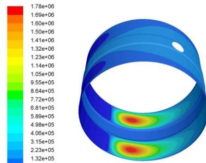
Figure 2: Pressure distribution (Pa) on bushing surface
