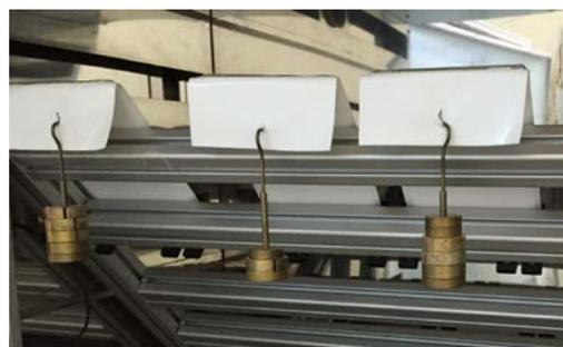
Figure 1: Samples with weight hung from the top part of backsheet.
