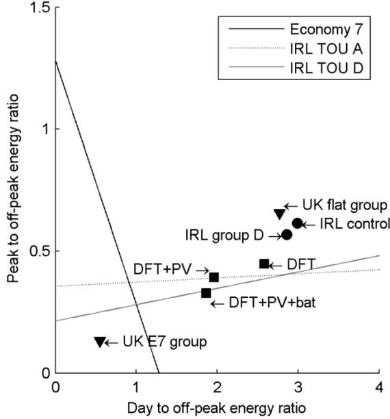
Figure 2. Energy-ratios for groups in relation to lines that indicate values that would produce no change in cost for three types of time-of-use pricing.
