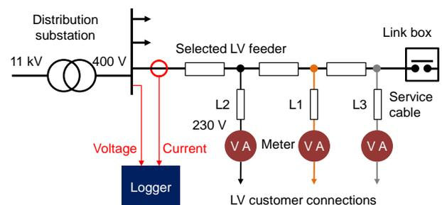
Fig. 2 LV feeder measurement configuration
