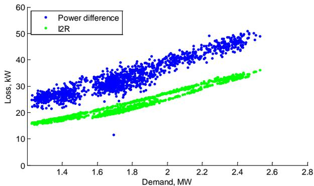
Fig. 8 HV feeder 1 loss vs. load
