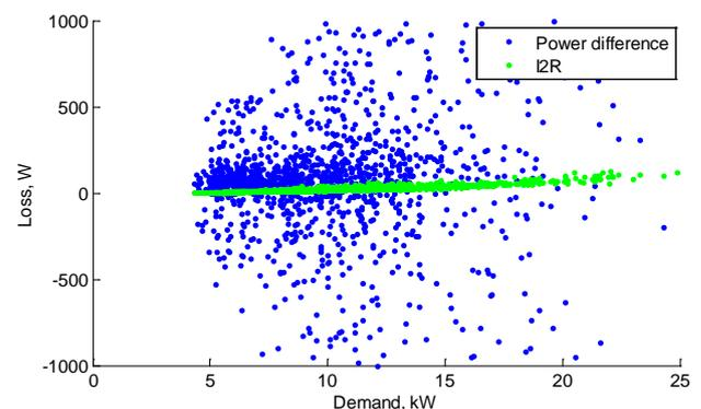
Fig. 7 Pilot trial LV feeder loss vs. load
