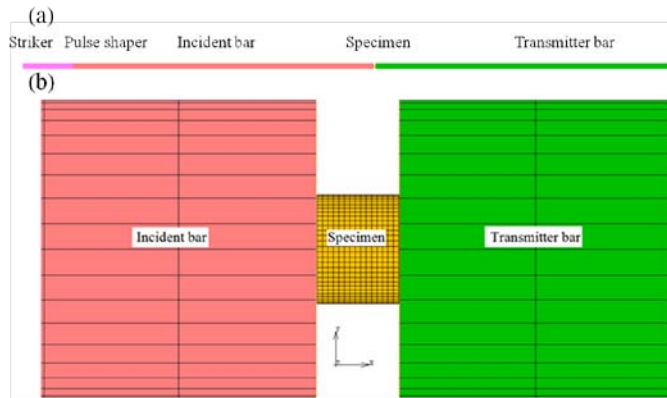
Figure 3: FE model of the SHPB experiment (a) and zoomed part with specimen tested (b)
