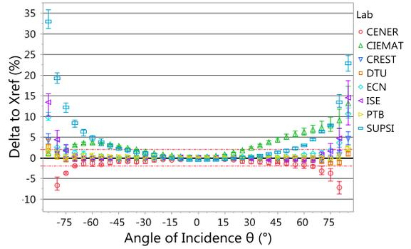
**Figure 3:** Plot showing the difference between each lab's measurement and the reference value  $X_{ref}$ . The error bars show each lab's max and min difference to  $X_{ref}$ . The red dashed reference lines are drawn at  $\pm 2\%$ .
