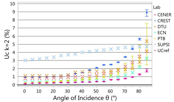
**Figure 1:** Expanded uncertainty from six laboratories as a function of AOI. The expanded uncertainty of the reference ( $UC_{ref}$ ) is also shown. Labs providing a single uncertainty value at each angle are noted with an 'x' whereas labs with uncertainty specific to each DUT are noted with dots and range bars.
