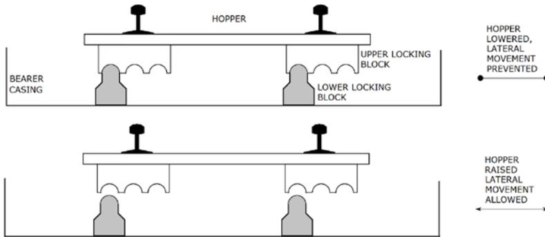
**Figure 3: Passive locking elements of each actuator-bearer unit**
