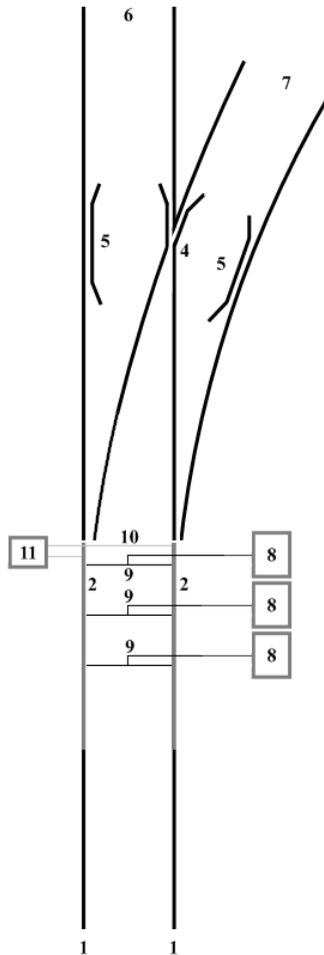
**Figure 1: Proposed high-availability stub-switch concept with redundant actuation paths. 1 (Black, Bold) Stock Rails; 2 (Grey, Bold) Moveable Switch Rails; 4 Common Crossing; 5 Check Rails; 6 Straight Route; 7 Turnout Route; 8 Multi-Channel Actuators; 9 (Black) Drive Rod and Linkages ; 10 Detection Rods ; 11 Blade Position Detection and Feed-back Unit. Reproduced from (9)**
