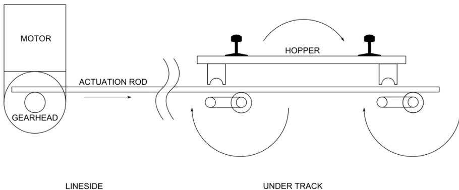
**Figure 2: Mechanical transmission elements of each actuator-bearer unit**
