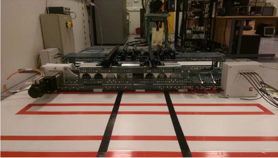
**Figure 8: 384mm scale actuator bearer in laboratory**
