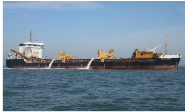
Figure 1 Sand Falcon whilst pumping water only (draghead raised)
