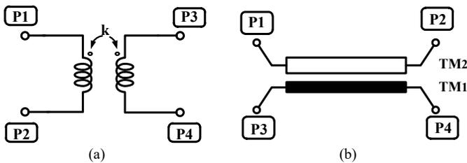
Fig.1. Schematics of (a) ideal coupled-inductors and (b) ideal four-port broad-side coupling line (BCSL).
