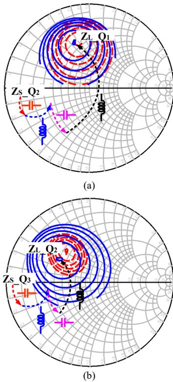
Fig.10. Inter-stage matchings for 3-stage PA (a) from Q<sub>1</sub> to Q<sub>2</sub> and (b) from Q<sub>2</sub> to Q<sub>3</sub>.
