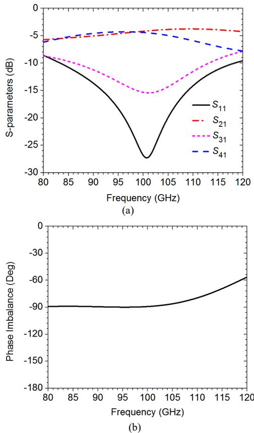
Fig. 7. Full EM-simulated results of proposed coupler with (a) S-parameters and (b) Phase imbalances.
