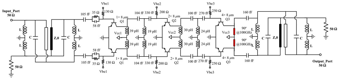
Fig.9. Circuit schematic of W-band balanced power amplifier with proposed quadrature coupler implementation in 0.13µm SiGe.
