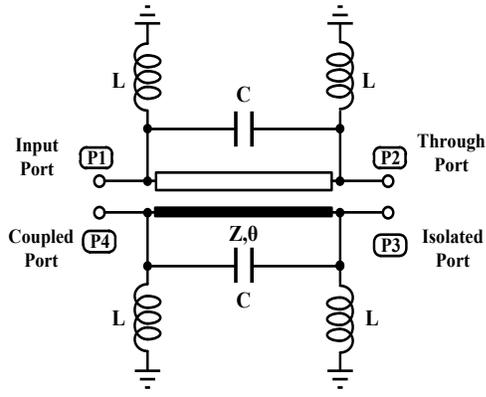
Fig.3. Schematics of proposed coupler with BCSL.
