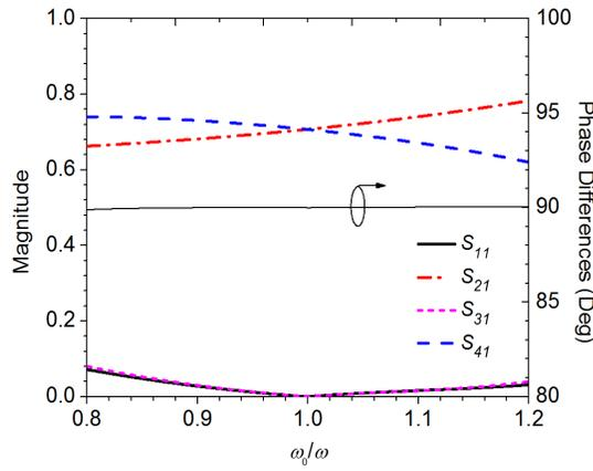
Fig.5. Theoretical results of proposed coupler with S-parameters and phase imbalances.
