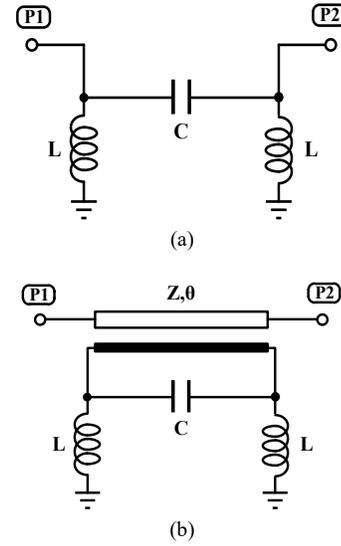
Fig.4. Half circuits of proposed coupler with BCSL (a) Even-mode and (b) Odd-mode.
