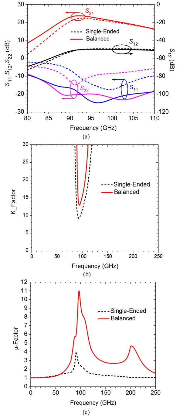
Fig. 12. Simulated results of (a) S-parameters (b) K-factor and (c)  $\mu$ -factor for the single-ended and proposed balanced PA.
