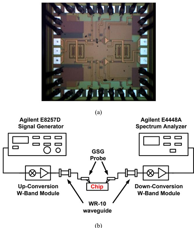
Fig.13. (a) W-band balanced PA with proposed quadrature coupler die photograph in 0.13- $\mu\text{m}$  SiGe. ( $0.8 \times 0.8 \text{ mm}^2$  including pads) (b) W-band PA measurement setup.
