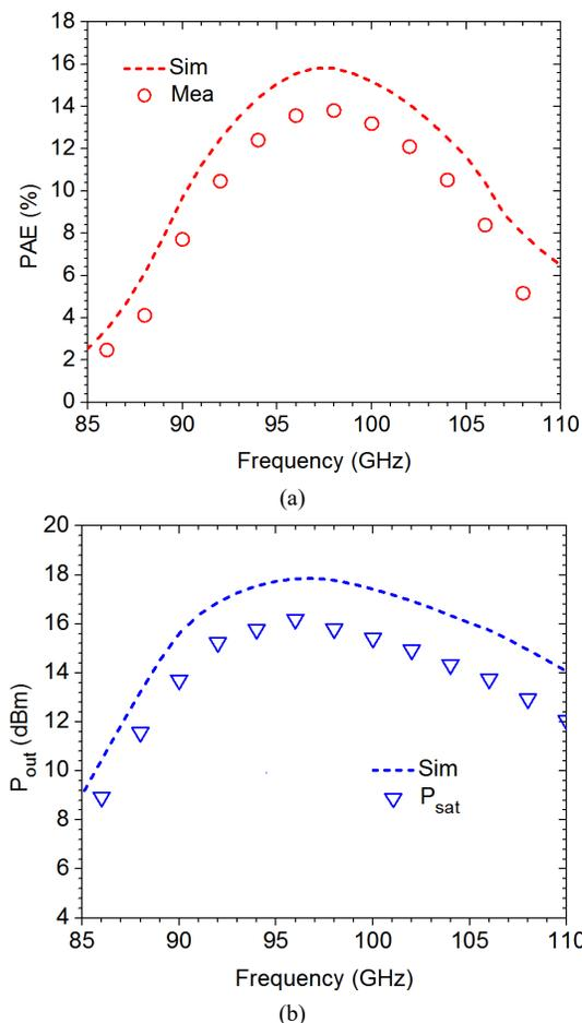
Fig.14. Simulated and measured (a) PAE and (b)  $P_{\text{sat}}$ ,  $OP_{1\text{dB}}$  versus frequency of balanced PA with proposed quadrature coupler.
