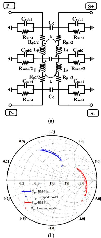
Fig.2. (a) Lumped-element model of BCSL (b) Comparison of four-port S-parameters of BCSL obtained using lumped-element model and HFSS EM simulations.
