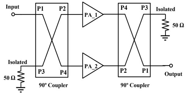
Fig. 8. Architecture of Balanced Power Amplifier.
