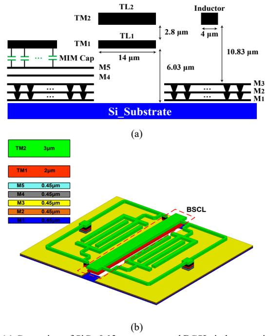
Fig.6. (a) Cross view of SiGe 0.13μm process and BCSL, inductors with M3 as ground plane (b) EM 3D layout of proposed quadrature coupler with BCSL.
