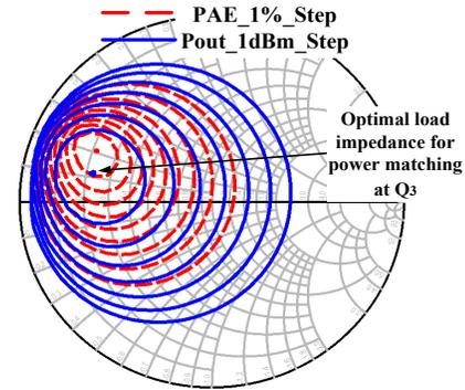
Fig.11. Simulated output power P<sub>out</sub> and PAE contours versus load impedance presented at Q<sub>3</sub>.
