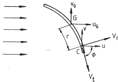
Fig. 2 Model of a textile fiber in an air flow:  $V_n = (u-u_G)\sin\phi + (v-v_G)\cos\phi + r(d\phi/dt)$
