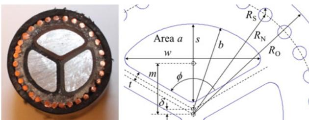
**Fig. 2** Sample cross-section of 3-core 95 mm<sup>2</sup> cable and dimensions
