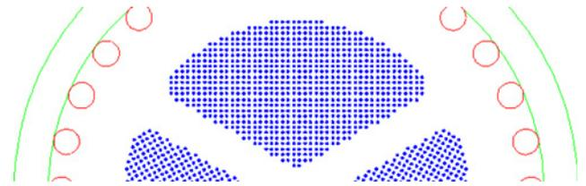
Fig. 3 Sub-conductor model of 3-core 95 mm<sup>2</sup> cable
