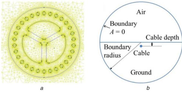
**Fig. 4** FEMM model showing of 3-core 95 mm<sup>2</sup> waveform cable
