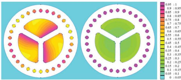
**Fig. 6** Relative current density from FEMM results, 350 Hz, 3-core 95 mm<sup>2</sup> cable
