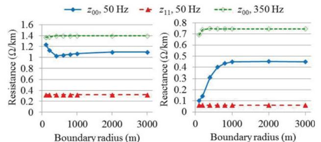
**Fig. 7** Positive ( $z_{11}$ ) and zero ( $z_{00}$ ) sequence impedances versus boundary radius, 3-core 95 mm<sup>2</sup> cable, ground resistivity of 100 Ωm, cable located 1 m below the surface
