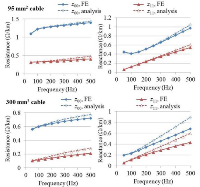
**Fig. 5** Positive ( $z_{11}$ ) and zero ( $z_{00}$ ) sequence impedances for 3-core 95 and 300 mm<sup>2</sup> cables
