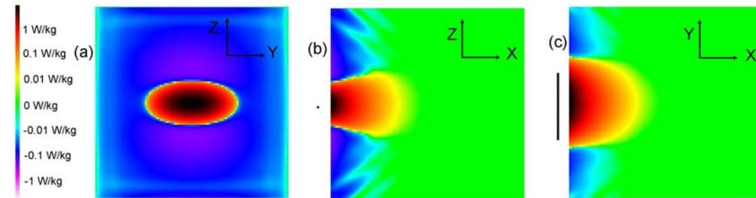
**Figure 6.** The difference in SAR with pin compared to without pin. (Figure 5 minus Figure 4); (a) is on the front surface of the phantom; (b) and (c) are the two cuts to the back of the phantom through the centre of the cube. NB The pin is included in (b) and (c).
