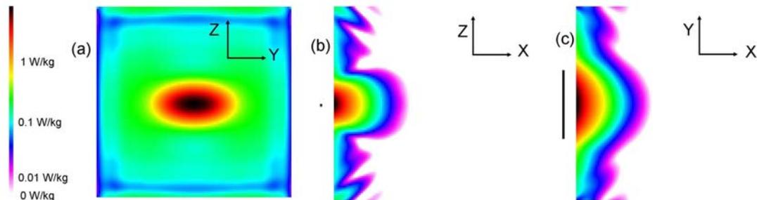
**Figure 5.** The SAR in Phantom 1 with  $0.42\lambda$  pin. (a) is on the front surface of the phantom. (b) and (c) are the two cuts to the back of the phantom through the centre of the cube. NB The pin is included in (b) and (c).
