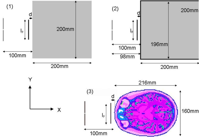
**Figure 1.** Orientation and geometry of dipole pin and head.
