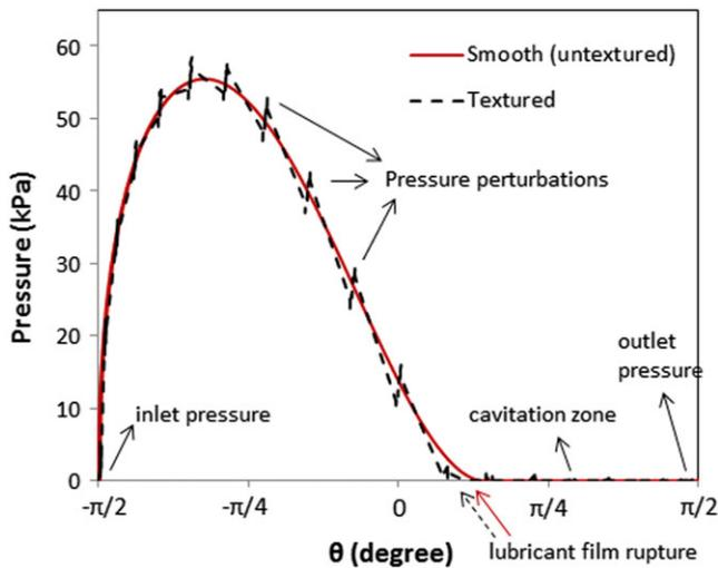
**FIGURE 9** Pressure distribution in the centre plane for 1.4-kg load condition [Colour figure can be viewed at [wileyonlinelibrary.com](http://wileyonlinelibrary.com)]
