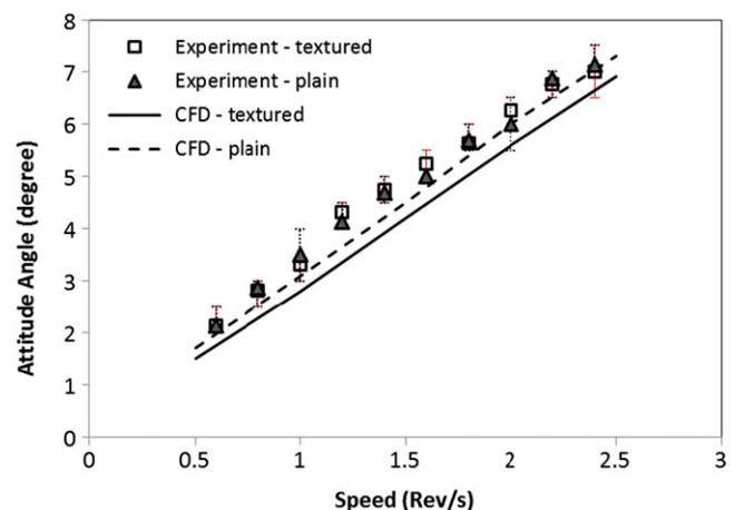
**FIGURE 8** Changes in attitude angle over a range of speeds for a load of 0.8 kg (CFD and experimental results). CFD indicates computational fluid dynamics [Colour figure can be viewed at [wileyonlinelibrary.com](http://wileyonlinelibrary.com)]
