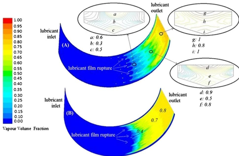
**FIGURE 10** Contours of vapour volume fraction for (A) textured and (B) untextured journal bearing for a load of 1.4 kg [Colour figure can be viewed at [wileyonlinelibrary.com](http://wileyonlinelibrary.com)]
