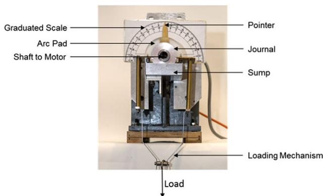
**FIGURE 1** Experimental rig [Colour figure can be viewed at [wileyonlinelibrary.com](http://wileyonlinelibrary.com)]
