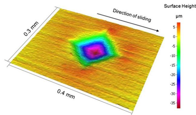
**FIGURE 3** An individual surface texture taken by an infinite focus microscope [Colour figure can be viewed at [wileyonlinelibrary.com](http://wileyonlinelibrary.com)]
