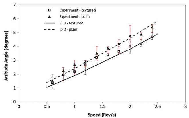
**FIGURE 7** Changes in attitude angle over a range of speeds for a load of 1.4 kg (CFD and experimental results). CFD indicates computational fluid dynamics [Colour figure can be viewed at [wileyonlinelibrary.com](http://wileyonlinelibrary.com)]
