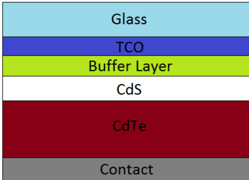
Figure 1 A schematic diagram of the CdTe solar cell structure showing the position of (from bottom to the top), the back contact, the CdTe absorber, the CdS window layer, the buffer layer, the TCO layer, and the glass substrate.
