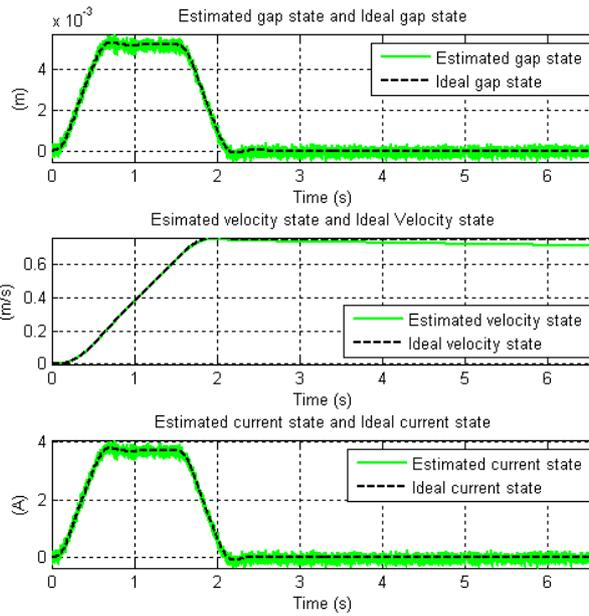
Fig. 8 State estimation with vertical acceleration measurement
