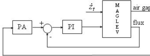
Fig. 4 Classical controller implementation with flux inner loop feedback
