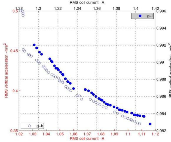
Fig. 5 Pareto front of controllers for  $(z_t - z), b$  (empty dots) and  $(z_t - z), i$  (dark dots)
