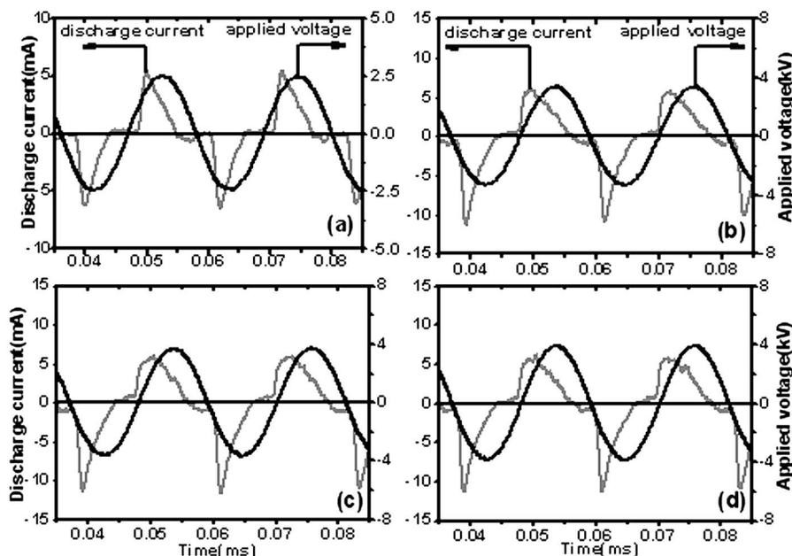
FIG. 3. Typical wave forms of the discharge voltage and current corresponding to the patterns in Fig. 2 with a fixed helium flow value of  $0.38 \text{ m}^3/\text{h}$  and at a peak applied voltage of (a) 2.5 kV, (b) 3.4 kV, (c) 3.7 kV, and (d) 4.0 kV.
