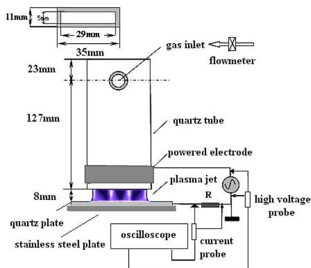
FIG. 1. (Color online) Experimental setup of the APPJ.
