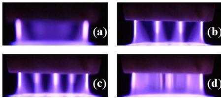
FIG. 2. (Color online) Formation process of the regular self-organized patterns with a fixed helium flow value of  $0.38 \text{ m}^3/\text{h}$  and at a peak applied voltage of (a) 2.5 kV, (b) 3.4 kV, (c) 3.7 kV, and (d) 4.0 kV.
