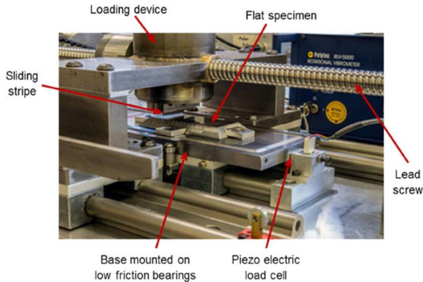
Figure 2. Detailed view of the contact in the floating plate arrangement. [Colour figure can be viewed at [wileyonlinelibrary.com](http://wileyonlinelibrary.com)]
