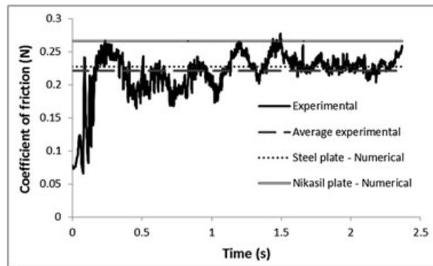
Figure 16. Coefficient of friction variation (experimental vs numerical).
