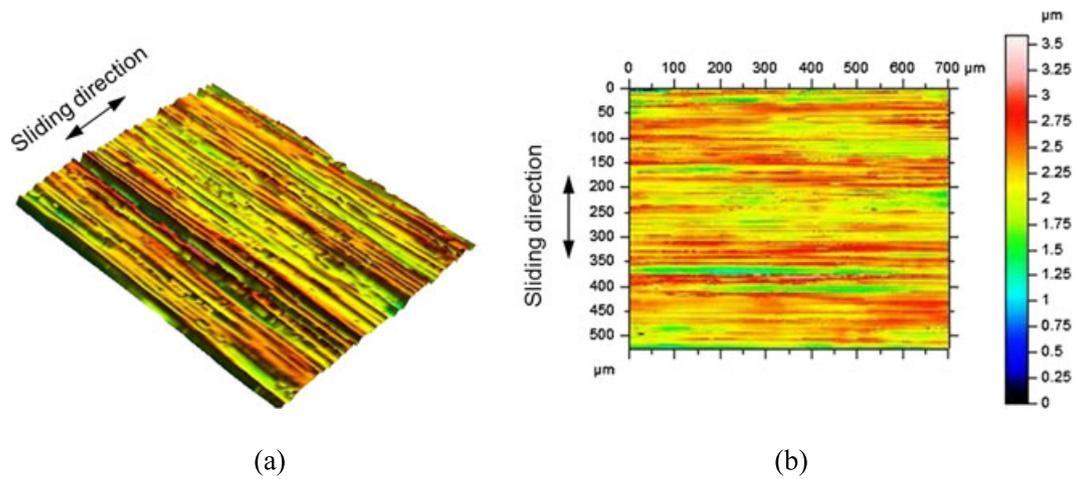
Figure 8. (a) 3D and (b) 2D view of the measured Ni-SiC plate surface. [Colour figure can be viewed at [wileyonlinelibrary.com](http://wileyonlinelibrary.com)]
