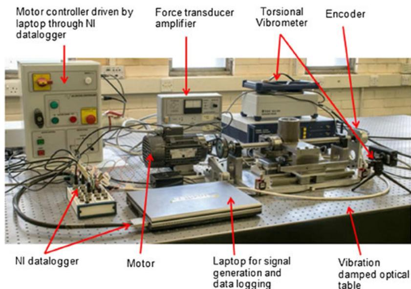
Figure 1. The precision sliding tribometer. [Colour figure can be viewed at [wileyonlinelibrary.com](http://wileyonlinelibrary.com)]
