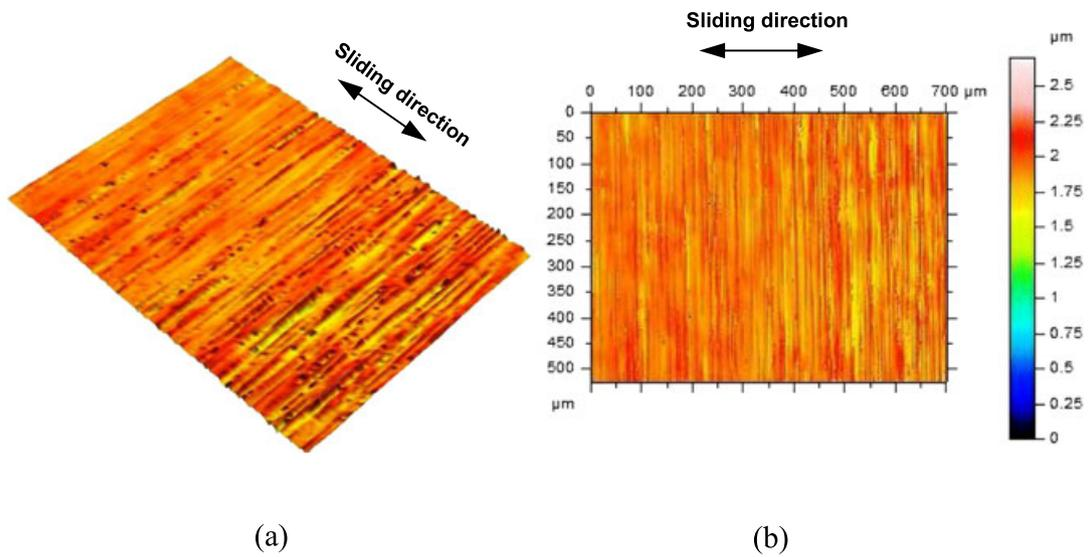
Figure 7. (a) 3D and (b) 2D view of the measured steel plate surface. [Colour figure can be viewed at [wileyonlinelibrary.com](http://wileyonlinelibrary.com)]
