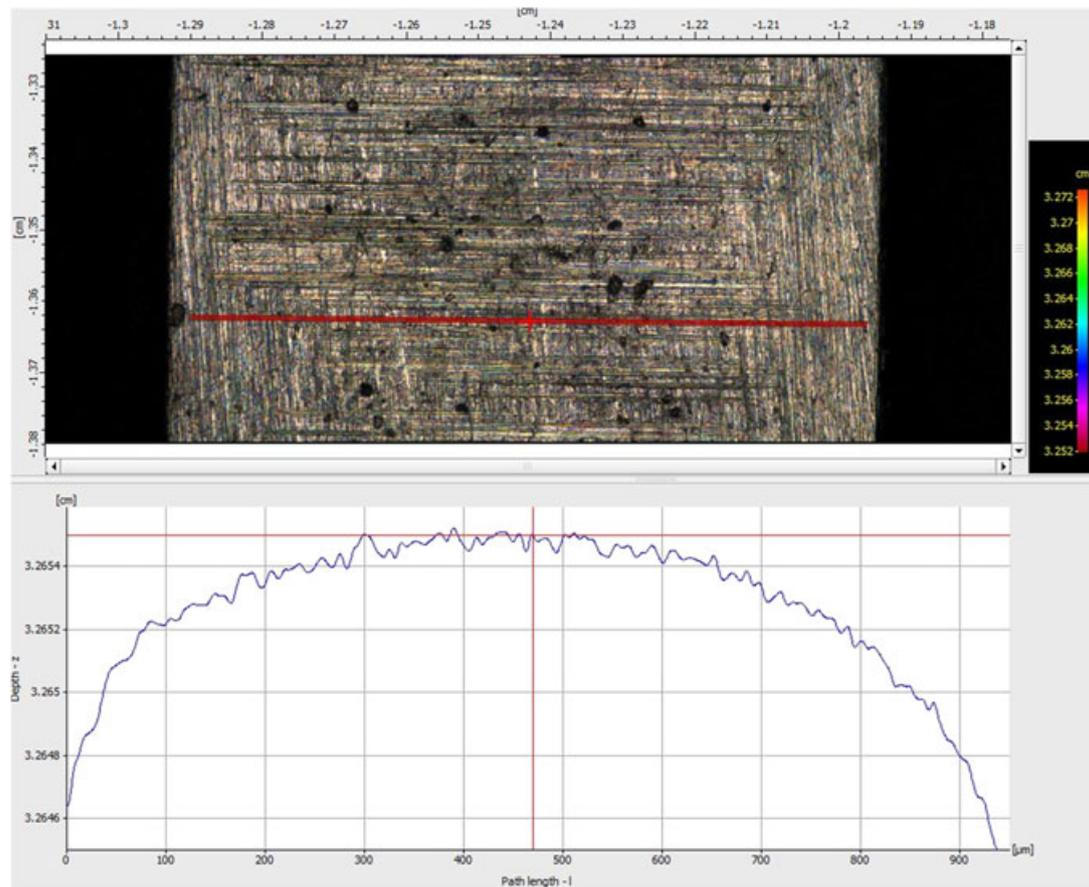
Figure 3. The parabolic profile of the sliding strip contact face through optical microscopy. [Colour figure can be viewed at [wileyonlinelibrary.com](http://wileyonlinelibrary.com)]
