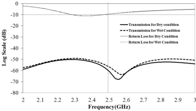
FIGURE 6 Simulated  $S_{21}$  (dB) and  $S_{11}$  (dB) results for the 4-layered Human torso model with antennas at front and back at 2.5 GHz
