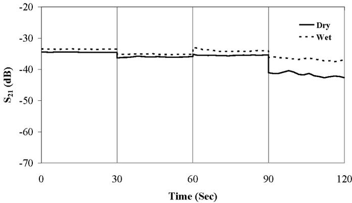
FIGURE 7 Measured  $S_{21}$ (dB) Between Waist-to-Chest worn antennas on the body with changes in posture (Frequency  $f=0.9$ GHz, 0-30s Standing Straight, 30-60s Torso Left, 60-90s Torso Right, 90-120s Bending Forward)
