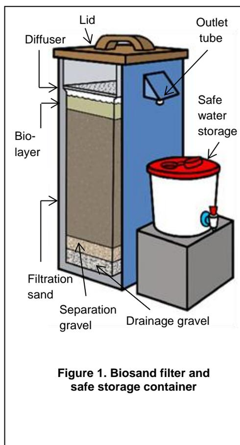
Figure 1. Biosand filter and safe storage container
