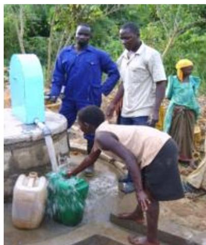
**Photograph 2. The fully covered rope pump model used in Uganda until 2011.**
