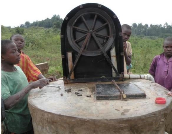
**Photograph 1. A section through the fully covered rope pump, designed only for a hand dug well.**
