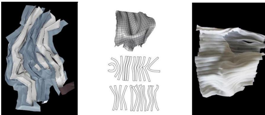
Fig. 7, 8, 9. First tests of unfolding a shape (from left to right: unfolding by Ivy plug-in for mesh analysis, self-coded unrolling, sewn prototype of the unrolling).
