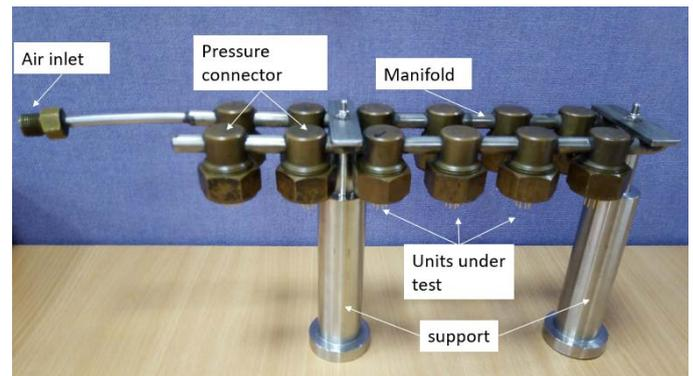
Fig. 3 Photograph of the sensors mounted on the manifold
