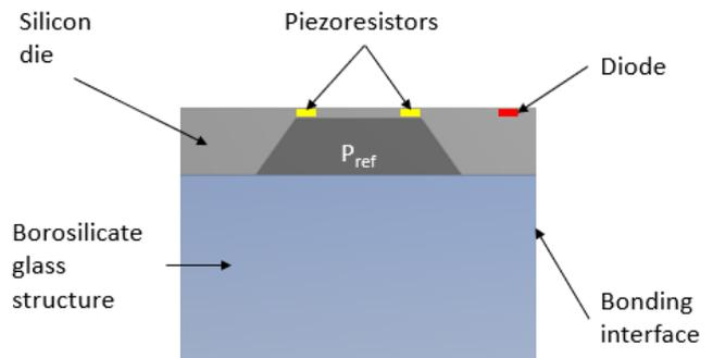
Fig. 1 The basic sensing element (SE) consisting of the silicon die bonded to a borosilicate glass structure
