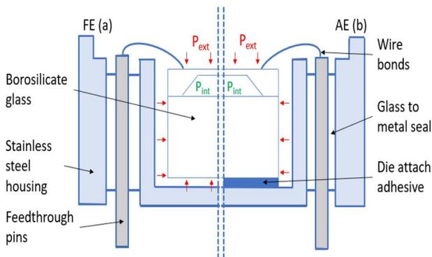
Fig. 2 Schematic of (a) “Floating Exposed” (FE) and (b) “Attached Exposed” (AE) packaging configurations
