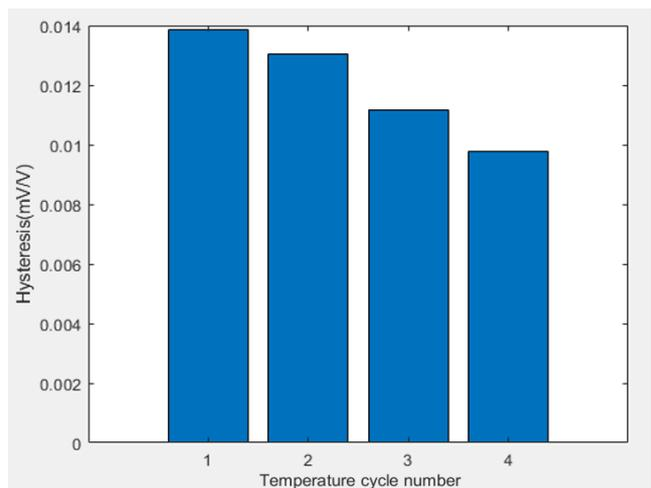
Fig. 9 Thermal hysteresis for SE #9 packaged in the AE configuration subjected to four thermal cycles
