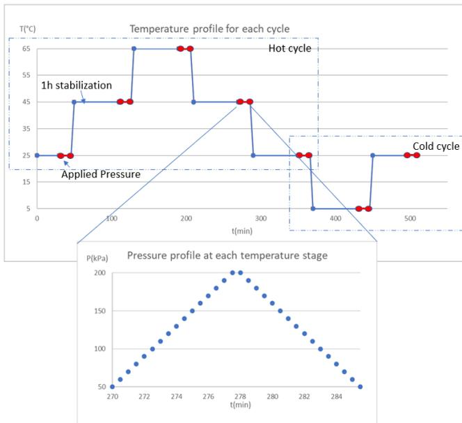
Fig. 4 Temperature and pressure profile for the first cycle
