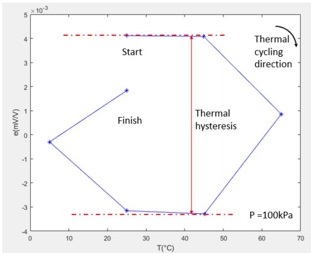
Fig. 6 Fitting error as a function of temperature for a FE packaged sensor (#9) at 100 kPa absolute pressure
