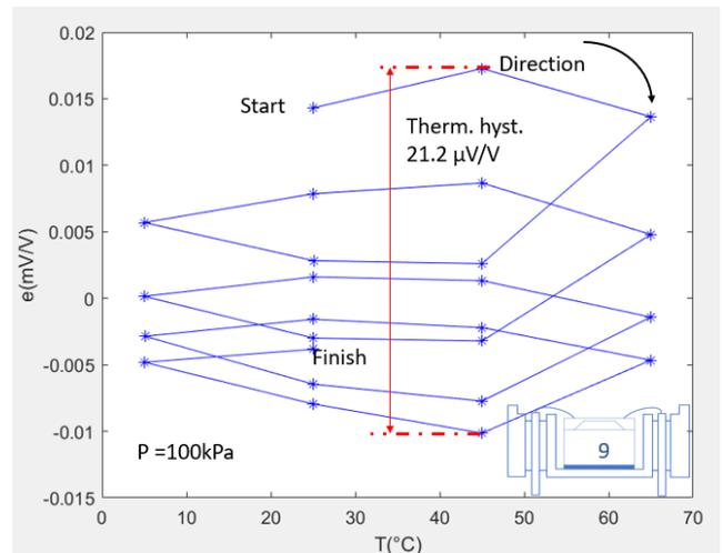
Fig. 8 Thermal cycle fitting error plots for AE test sample #9
