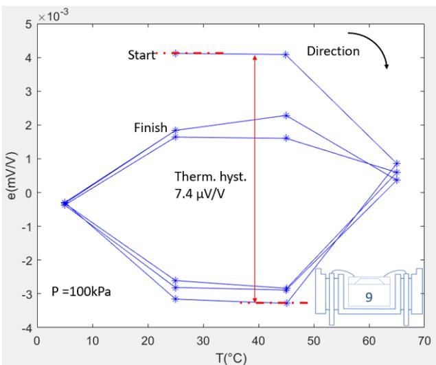
Fig. 7 Thermal cycle fitting error plots for FE test sample #9
