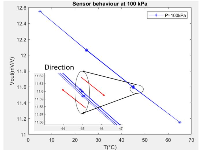
Fig. 5 Normalized bridge voltage output raw data for an FE package at 100 kPa for three 5 to 65°C cycles
