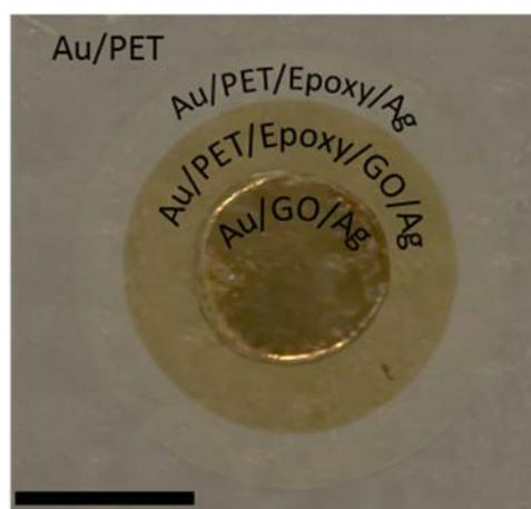
**Supplementary Fig. 2** | **Metal-GO-metal sandwich membrane device.** Photograph of one of our metal-GO-metal sandwich membranes attached to the PET sheet (step 2 in supplementary Fig. 1). Scale bar: 6 mm. This was further attached onto another plastic disc for sealing the metal container for gravimetric testing.
