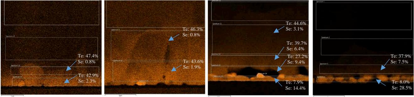
Fig. 1. Compositional maps for CST films produced with CdSe films of several thicknesses (150, 300, 1000, and 1500 Å from left to right).
