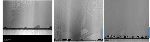
Fig. 3 STEM images for three CdSe thicknesses (300, 1,000, and 1,500 Å) (left to right) showing variations in the grain structure.
