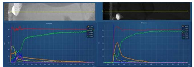
Fig. 4 EDS line scan results for two CST films (CdSe 1000-Å-left and 1500-Å-right) produced at a CdCl<sub>2</sub> HT temperature of 430 °C
