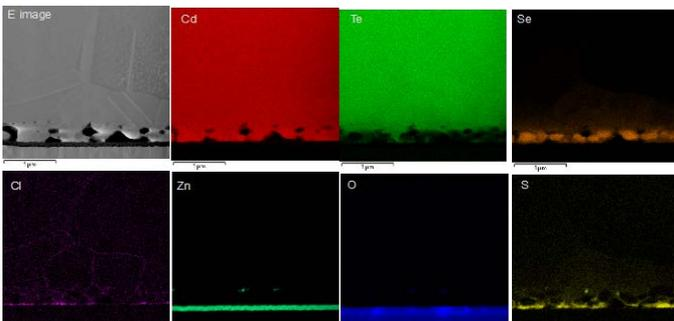
Fig. 2 EDS elemental mapping for a CST film produced with CdSe with 1500 Å thickness.
