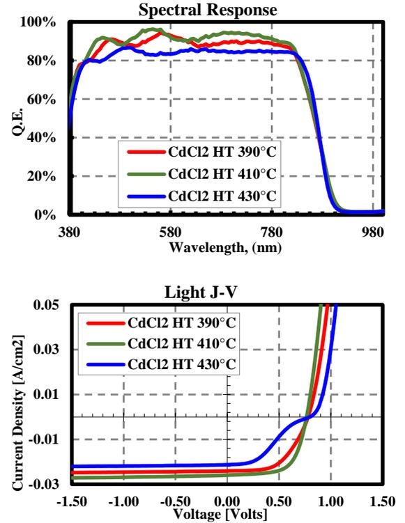
Fig. 6 SR and Light JV for three devices fabricated with 1000 Å thick CdSe and annealed at different  $CdCl_2$  temperatures (390 to 430 °C).
