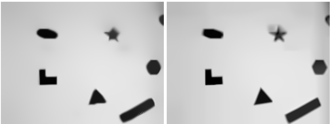
(g) NLM Filter \tilde{x}_{s,n} , n = mT , PSNR = 25.85dB, \lambda=5.25e-5 (h) BM3D Filter \tilde{x}_{s,n} , n = mT , PSNR = 26.38dB, \lambda=1.3e-4
