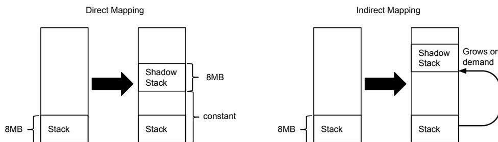
Figure 3.2.: Shadow stack designs – mapping options
