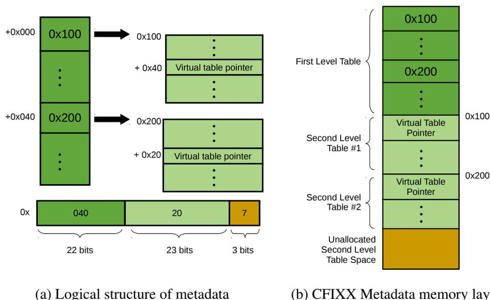
Figure 5.2.: Metadata design illustrated. Figure 5.2a shows how a pointer is broken into two indexes into the top level and second level table. The entry for the top level table points to the second level table. Figure 5.2b shows how all the tables are laid out in the protected data region. The top level table is allocated first, then all second level tables are allocated on demand.
