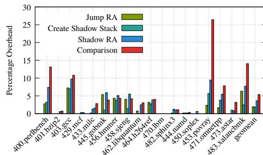
Figure 3.8.: Overhead breakdown for a compact register configuration
