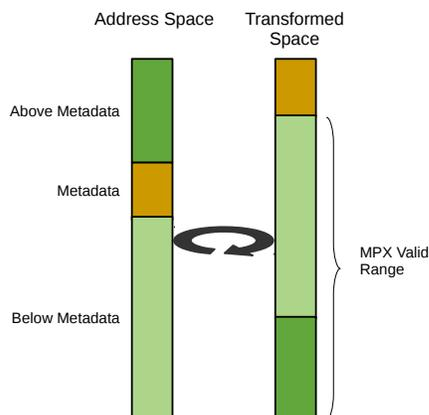
Figure 5.3.: Address space rotation for MPX checks
