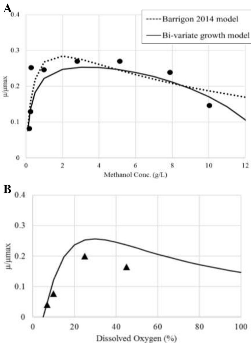
Figure 7: Bi-variate growth model approximations superimposed on other works; Black line: Bi-variate growth Equation 6 [This work] utilizing model parameters from Table 3; Black Circles: Empirical data from [Barrigon 2015]; Dotted line: Non-monotonically increasing function from [Barrigon 2015]; Black Triangles: Empirical Data from [Ponte 2016]
