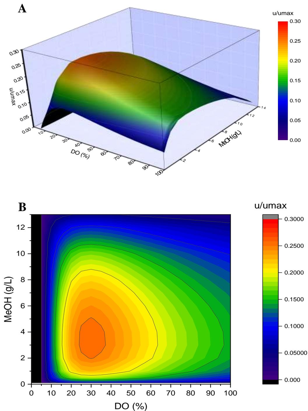
Figure 5: Surface plot of bivariate *Pichia* growth model against methanol and dissolved oxygen; A) 3-dimension surface plot and B) 2-dimensional projection of surface; black lines indicate culture conditions that theoretically would result in equivalent growth rates. Values for this image were calculated using Excel (Microsoft, 2013) and the images generated using Origin Imaging Software (OriginLab Corp, 2018)
