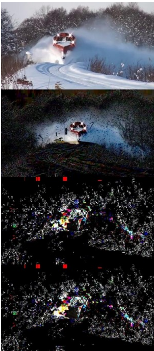
Figure 4.3. Results of Snowtrain Video. Row 1 is the original frames. Row 2 is the results of RegPCA, Row 3 is the result of RPCA with 10 iterations. Row 4 is 50 iterations of RPCA.
