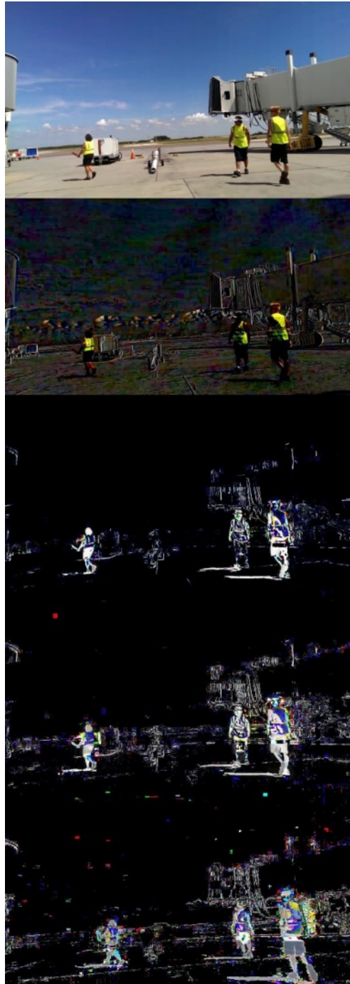
Figure 4.2. Results of Airport Video. Row 1 is the original frames. Row 2 is the results of RegPCA, Row 3 is the result of RPCA with 10 iterations. Row 4 is 50 iterations and Row 5 is 10000 iterations of RPCA.
