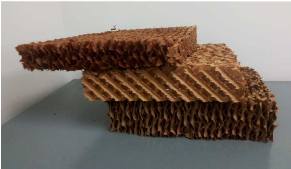
Figure 3. 1 Cellulose pads of thickness 2, 3 and 4 inches
