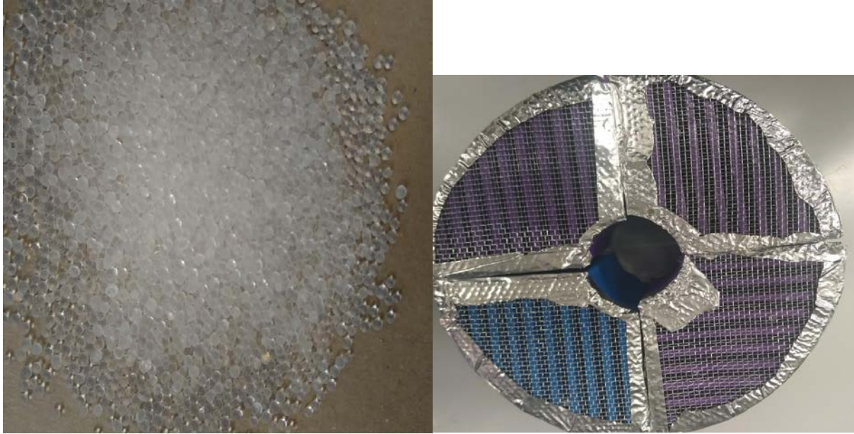
Figure 3. 2 Silica gel beads and silica gel beads impregnated into the cassettes
