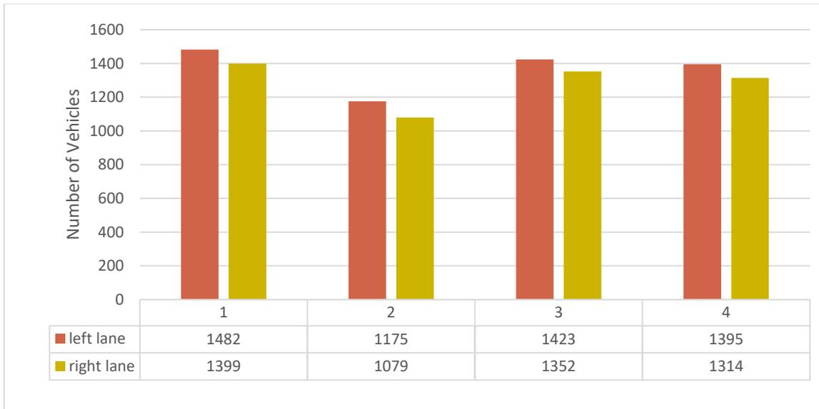
Figure 5.5 Comparing the number of vehicles on each lane at four different sections of the road at Patience 5 Seconds
