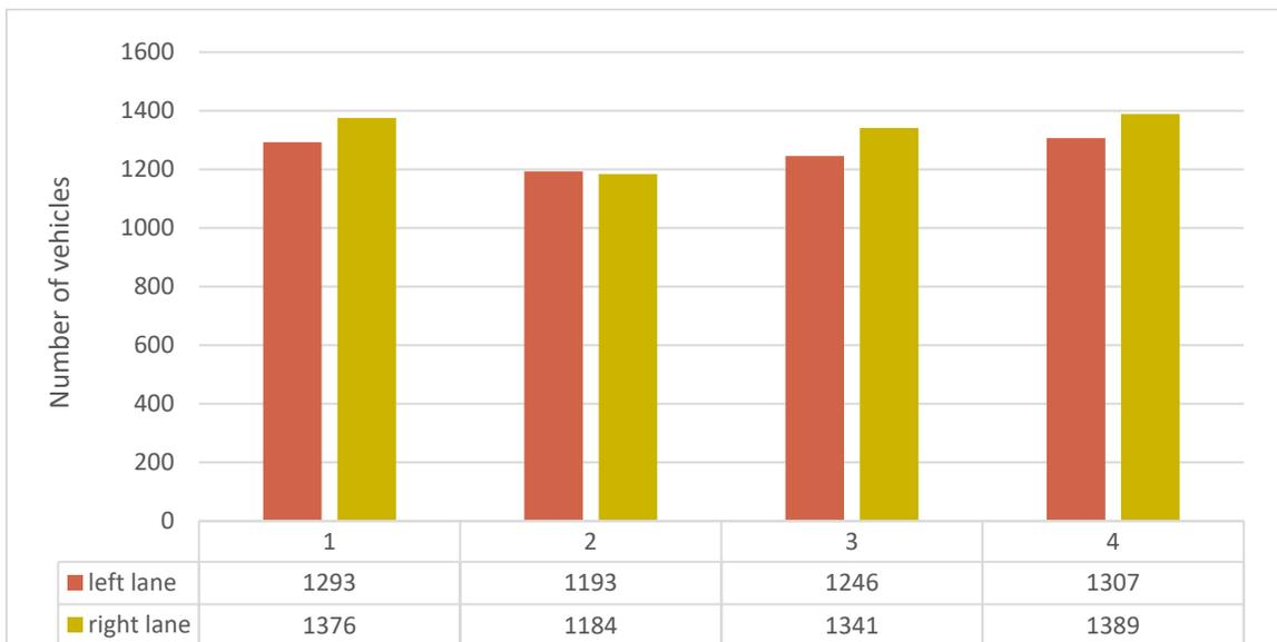
Figure 5.6 Comparing the number of vehicles on each lane at four different sections of the road at Patience 10 Seconds
