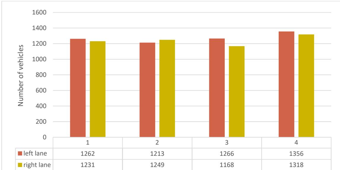
Figure 5.7 Comparing the number of vehicles on each lane at four different sections of the road at Patience 15 Seconds
