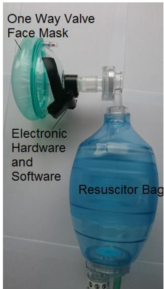
Figure 9.2: Complete LVR Adherence Prototype Electronic Software and Hardware
