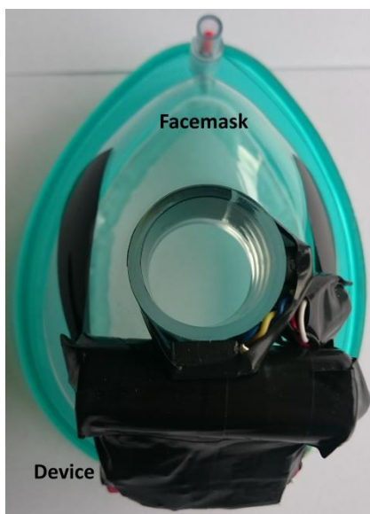
Fig. 3. Rear view of assembled prototype attached to facemask.
