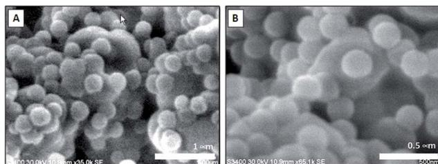
**Fig. 4** SEM images of PMA–SiNP decorated monoliths after being flushed with 100 mL of 0.1 M of PBS (A) and 100 mL of HCl at  $\text{pH} = 4.5$  (B). Both images were taken from Section II of the monolith (see Fig. 3).
