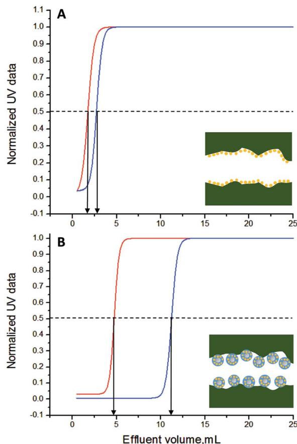
**Fig. 5** Best fit curves ( $R^2 > 0.99$  for all curves) for the extraction performed using myoglobin (in red) and the blue dextran (in blue) for the carboxylic acid functional monoliths (A) and the PMA–SiNP decorated monolith (B). Arrows indicating  $V_R$ . Yellow dots in cartoon represent carboxylic acid functions in surface modified monolith (A) and PMA–SiNP decorated monolith (B).
