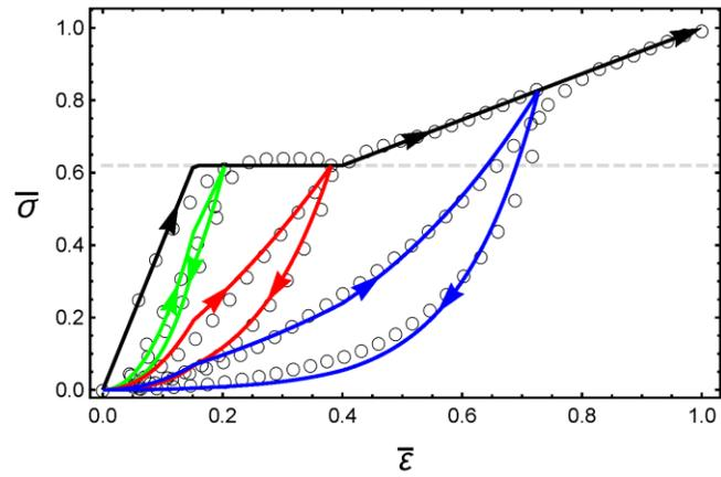
**Figure S1:** Comparison between the predictions of the proposed model in Eq. (S2) and the experimental results for a plaque subjected to multi-cyclic loading. The continuous curve and the circular markers correspond to the proposed model and experimental data, respectively.
