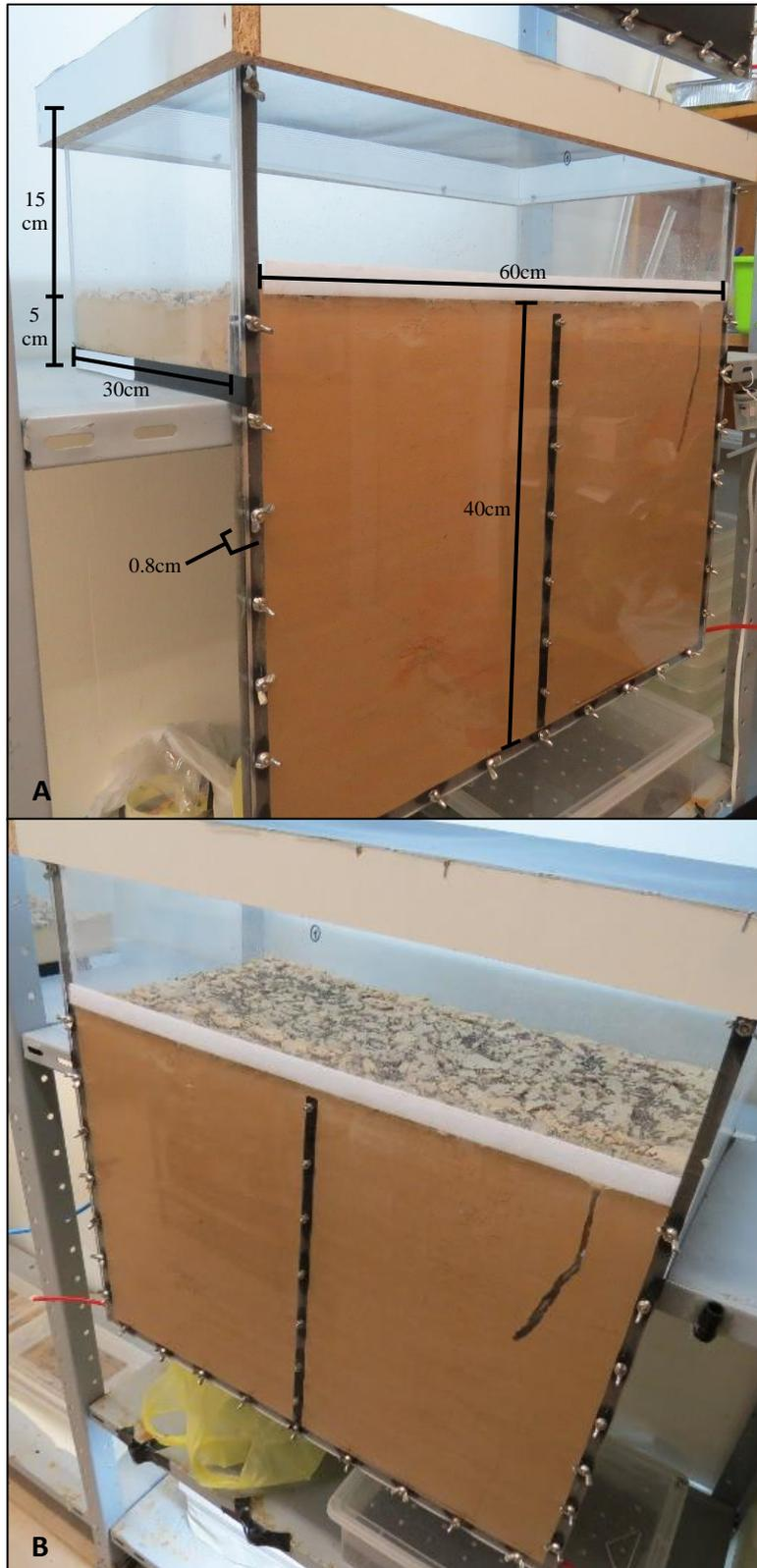
**Figure S2-6** – An informative view of Isopolis, exhibiting the dimensions and soil depth of the above- and belowground chambers (A), the surface-covering biological soil crust with *Haloxylon scoparium* litter scattered above, and a pair of isopods inside the burrow (B). The horizontal white stripe is a Velcro fastener for connecting the opaque front screen.
