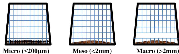
**Figure S2-2 - An illustration of the litter baskets design**
