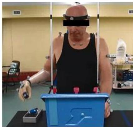
Figure 1. Setup for RCRT with clothespins positioned on middle horizontal rod. Both vertical rods shown, though only one is used during any test and the other is removed.
