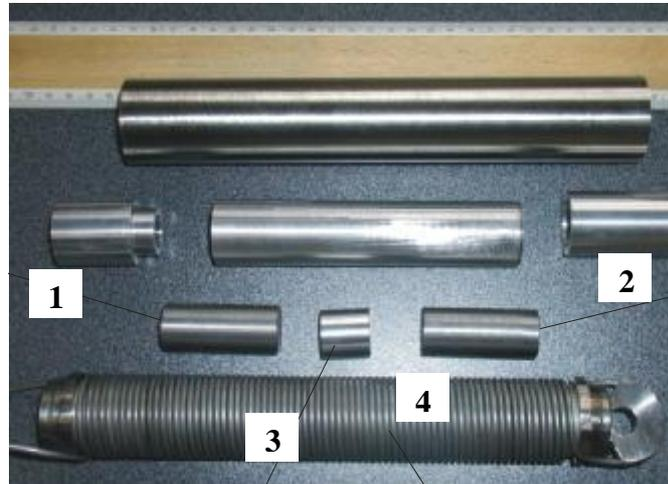
Figure 6 - Experimental device for RPV steel billets irradiation. (1 and 2 – RPV metal billets, 3 - capsule for neutron monitors, 4 – heater).
