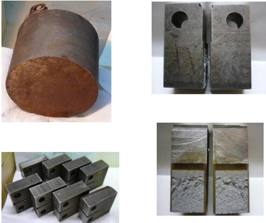
*Figure 2 - Steps of 1T-CT type specimens from 140 mm in diameter EPR RPV trepan manufacturing (left side) and testing.*
