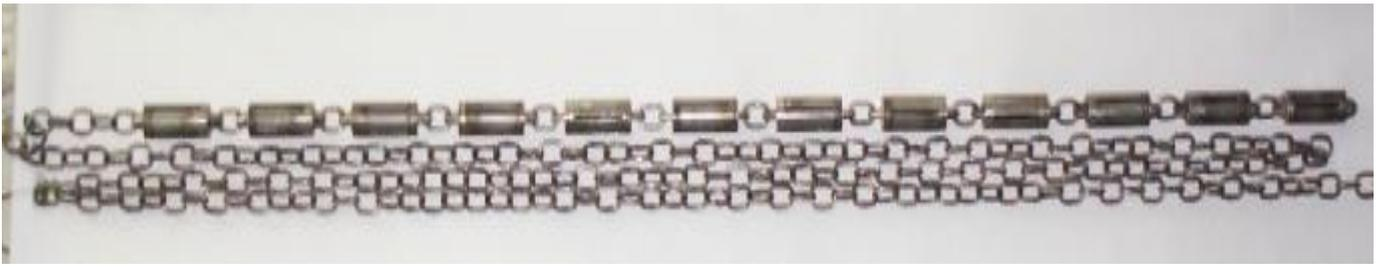
Figure 3 - Set of the perforated capsules with cylindrical billets inside.
