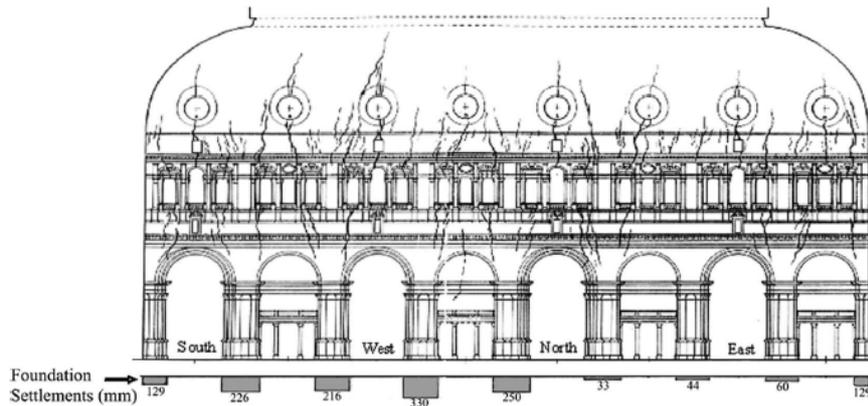
Figure 1 - Schematic of crack patterns and foundation settlements.
