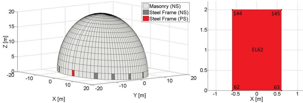
Figure 3 - Finite elements substructured mesh of the drum-dome system.
