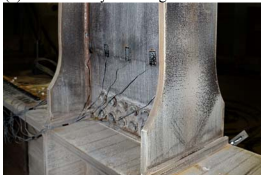
Figure 7 – Yielding and local buckling of the WF2 beam section at 4 and 5% rad story drift angle.
