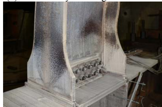
Figure 7 – Yielding and local buckling of the WF2 beam section at 4 and 5% rad story drift angle.
