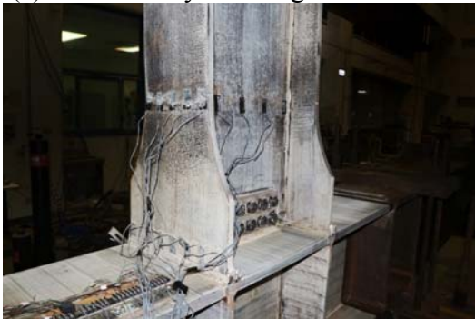
Figure 6 – Yielding and local buckling of the WF1 beam section at 4 and 5% rad story drift angle.
