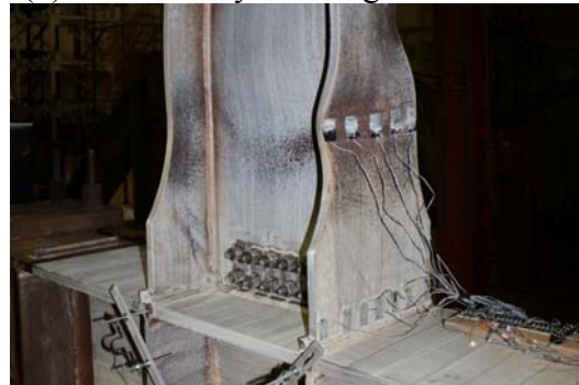
Figure 6 – Yielding and local buckling of the WF1 beam section at 4 and 5% rad story drift angle.
