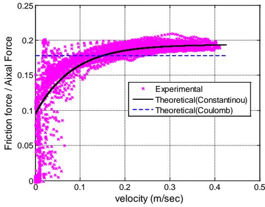
Figure 4 Friction coefficient vs. sliding velocity
