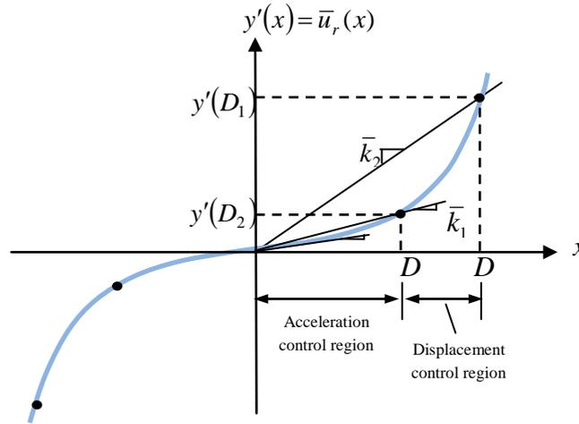
Figure 2 The normalized restoring force of the PFPI.
