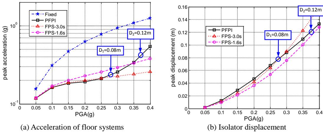
Figure 7 Average peak responses of various floor isolation systems subjected to the selected 10 ground motions.
