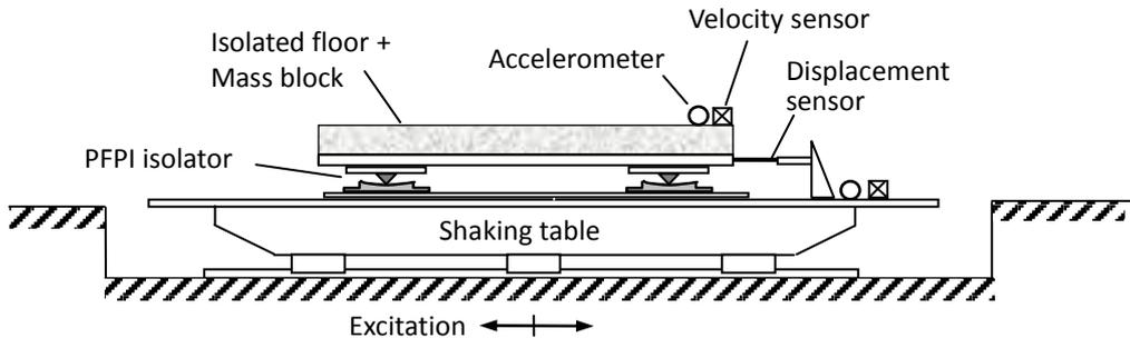
Figure 3 Setup of the hysteresis property test for the prototype PFPI-FIS.
