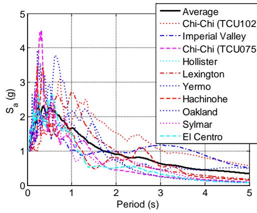
Figure 6 Acceleration response spectra of the selected 10 ground motions (5% damped).
