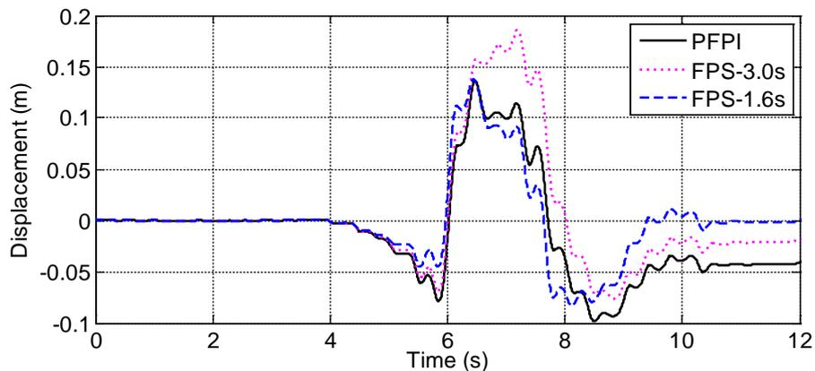
Figure 8 Comparison of isolator displacements (Imperial Valley earthquake, PGA=0.4g).
