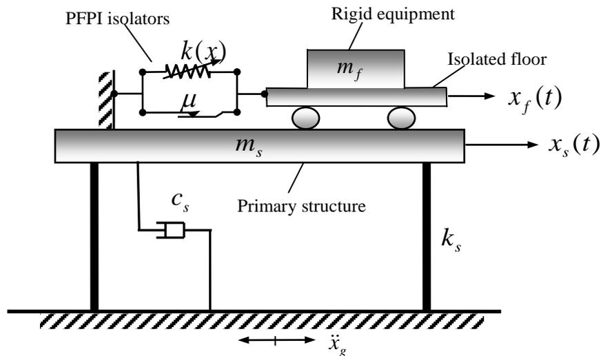
Figure 1. Mathematical model of a building with a PFPI floor-isolation system.
