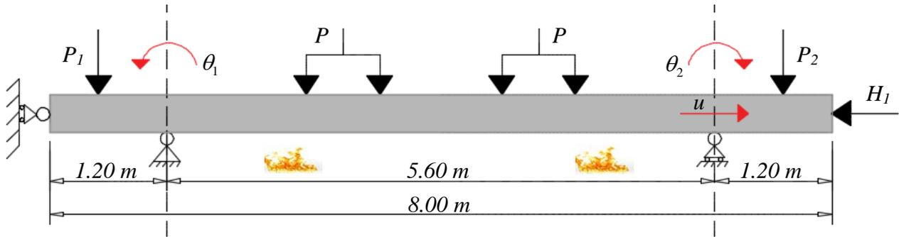
Figure 3 – The configuration of the physical specimen PS.
