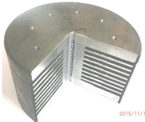
Figure 9 - Internal view of an ARB specimen after more than 200 cycles of loadings
