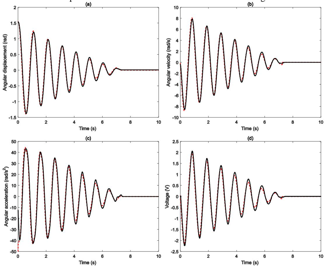
Figure 4 - measured (dashed line) simulated (solid line) (a) displacement, (b) velocity, (c) acceleration and (d) voltage for an initial condition of about  $\pi/2$  displacement in open circuit condition.
