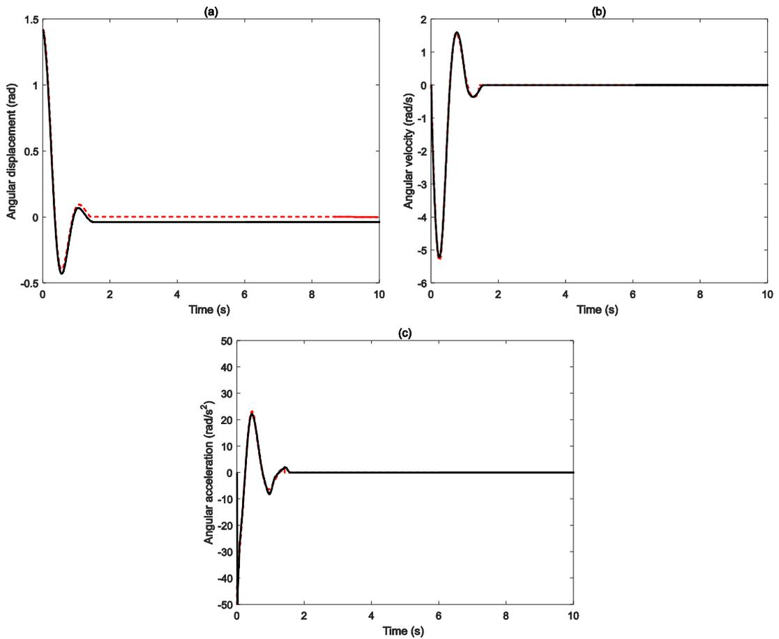
Figure 5 - measured (dashed line) simulated (solid line) (a) displacement, (b) velocity, (c) acceleration and (d) voltage for an initial condition of about  $\pi/2$  displacement in short circuit condition.
