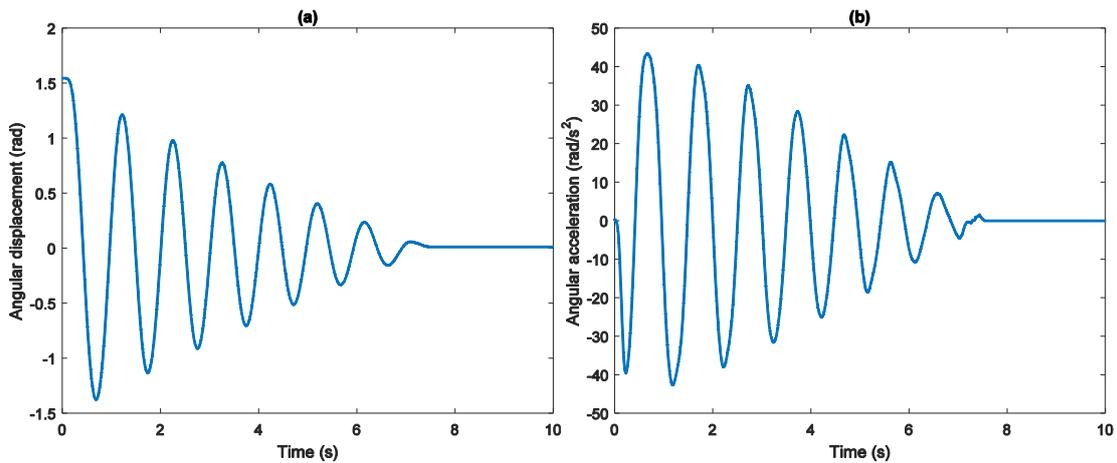
Figure 2 - time history of (a) angular displacement and angular acceleration for an initial displacement of about  $\pi/2$  radiant displacement.
