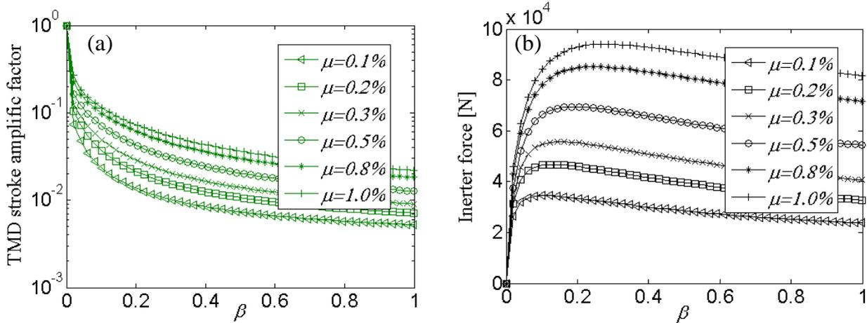
Figure 5- (a) Peak TMDI attached mass displacement normalised to the corresponding value for the classical TMD ( $\beta=0$ ), and (b) Peak inerter force developed for different values of inertance ratio  $\beta=b/M$  and attached mass ratio  $\mu= m_{TMDI}/M$ .
