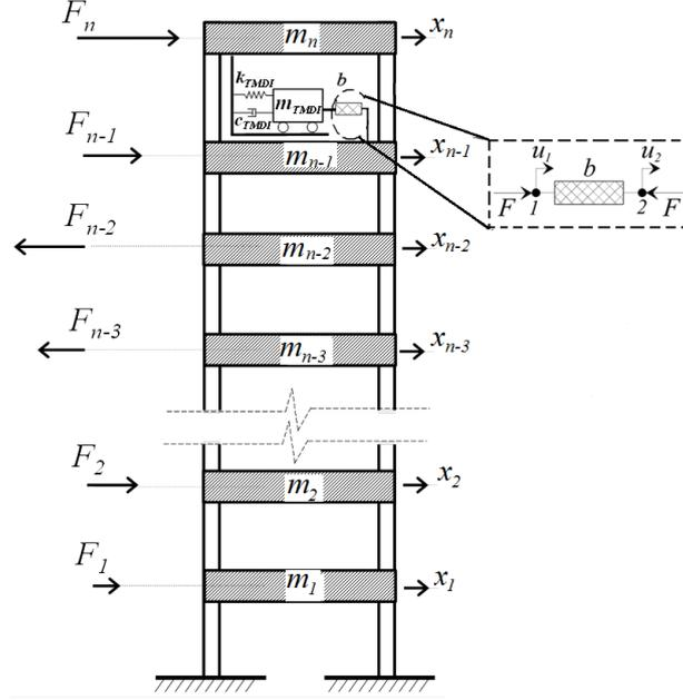
Figure 1 - Lumped-mass model of a tuned mass-damper-inerter (TMDI) equipped  $n$ -storey building subject to arbitrary (instantaneous) lateral wind forces and schematic representation of an inerter device subject to an external force  $F$ .
