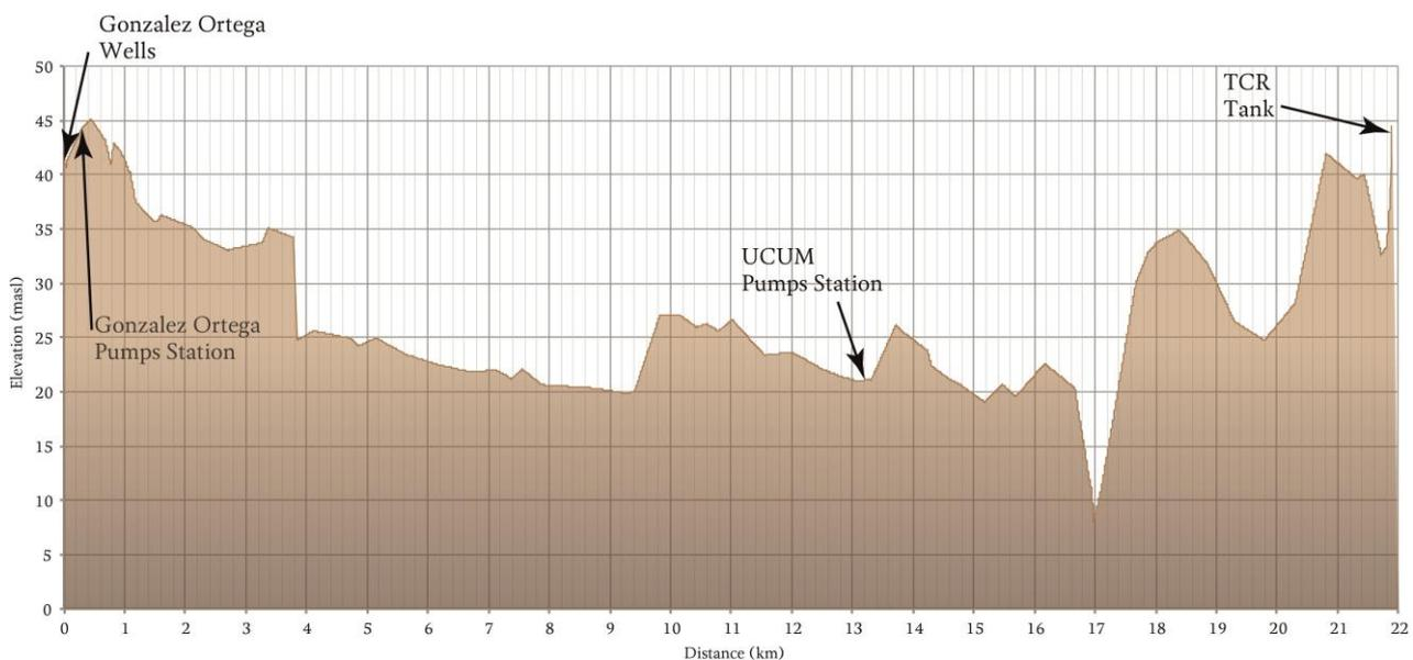
Figure 6. Piping profile with the location of the Pumps Stations and the TCR
